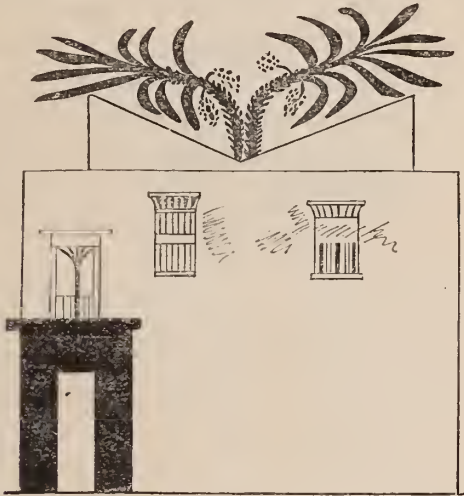
The mulquf for catching the wind.
